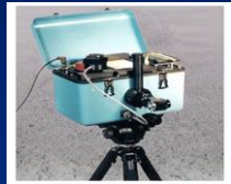
Model 102F FTIR (Fourier transform infrared) spectrometer
